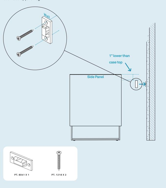
INSTALL ANTI-TIP BRACKET TO CASE.
